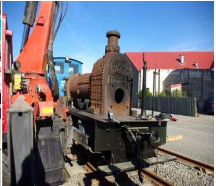
The boiler safely on the frame and wheels ready to be shunted into the depot.
