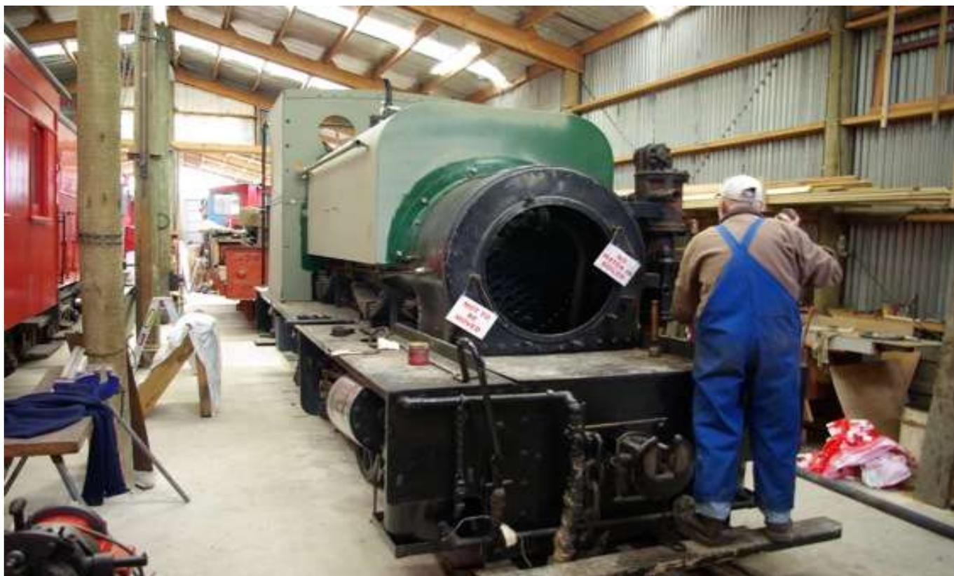
Member Frank Waller working on the Westinghouse pump of B 10. Great progress has been made on restoring B10 by a small group of members
